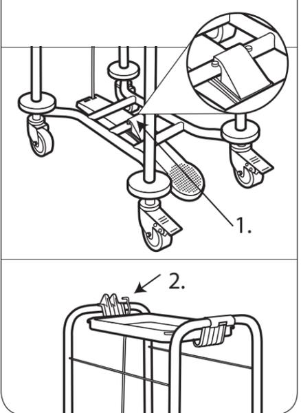
4. 1. Place lid lift lever under cart side frame close to bag frame.
