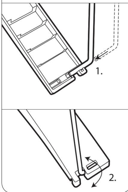
3. 1. Position the foot pedal underneath the cart, between the 2 anchor pins. Clip it on the central bar of the cart base.
