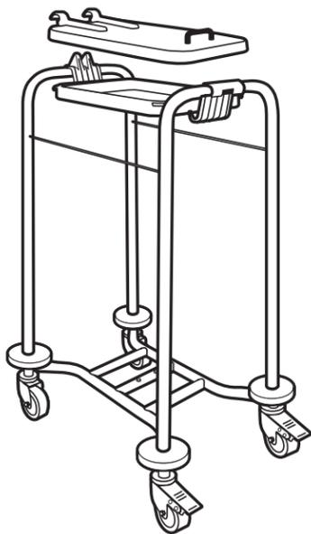
2. 1. Insert bottom end of the lifting rod in the slot of the foot pedal. It will be a tight fit.
